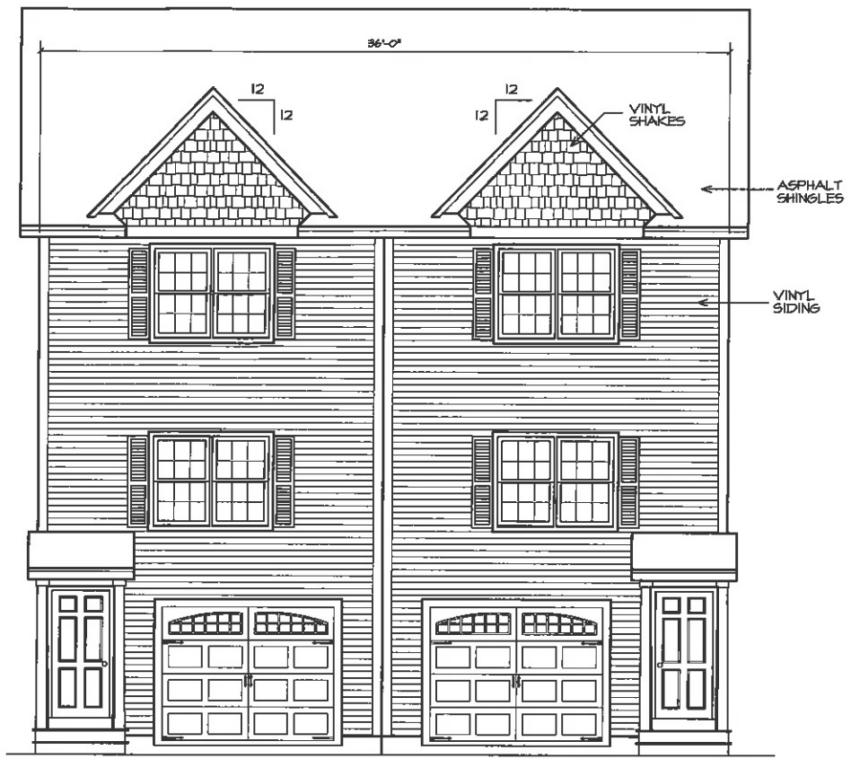
○ FRONT ELEVATION 2-UNIT
